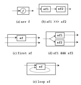
**Figure 1. Core Primitive Signal Functions**
